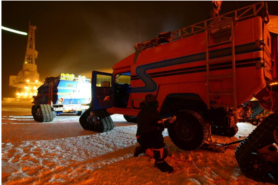
Team member, Rod Roddenberry prepares PTV2 for the ice by installing Mattracks at Oliktok Point. (Photo by Sherman Hon)
