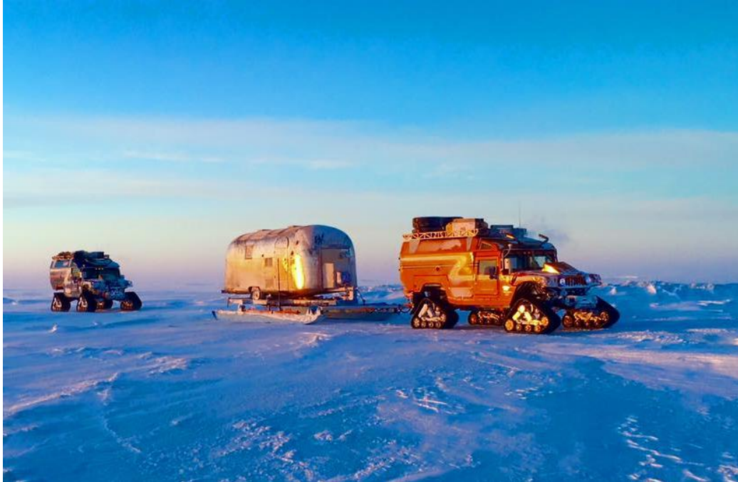
ZERO SOUTH Polar Traverse Vehicle convoy on the frozen Beaufort Sea. While in Alaska, the vehicles traveled a distance of 539 miles on paved roads, 514 miles on snow/gravel, 4 miles on solid ice road and 138 miles on sea ice (pictured above). (Photo by Richard Tukle)
