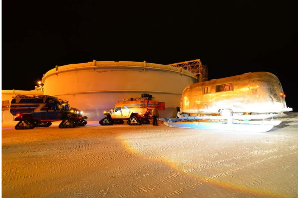
After many years of construction, the SnowStream was hitched to PTV2 and towed with ease for the first time. The vehicle generated 60kW towing across level, ungroomed snow surfaces. (Photo by Sherman Hon)
