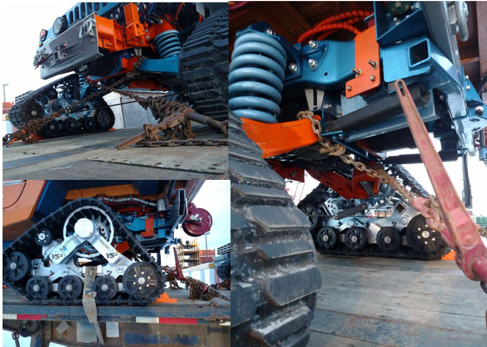
Observations made during three of eight vehicle transfers resulted in new methods for securing the ZERO SOUTH PTVs for transport. (Photos by Nick Baggarly)
