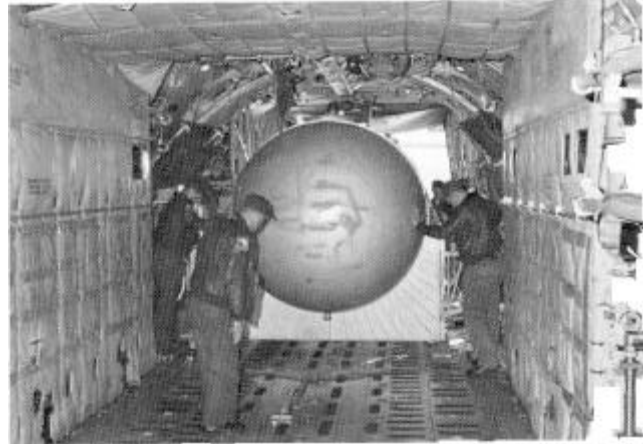
Both the mission and search planes were fitted with 3,500 gallon internal fuel tanks.
