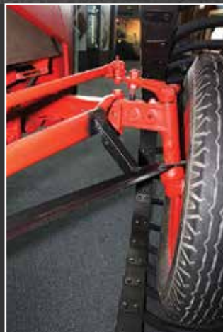
The restored tractor faithfully replicates the waratah standard which was added during the CTAE to strengthen the front wheel.
