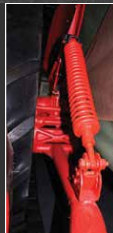
Close up showing the shock absorber system.
