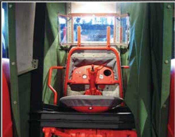
Image showing original windscreen from rear of tractor.
