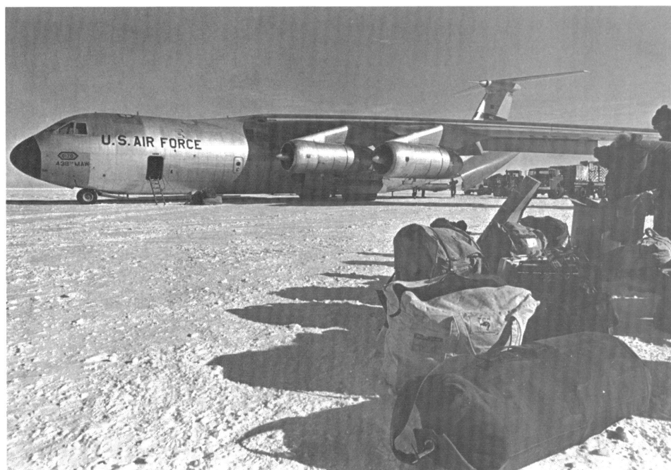
C-141 Starlifters, flown by the U.S. Air Force, began deploying people and priority cargo to Antarctica during Deep Freeze 67 . These wheeled airplanes, still used in U.S. antarctic programs, land on ice runways at McMurdo Station.
