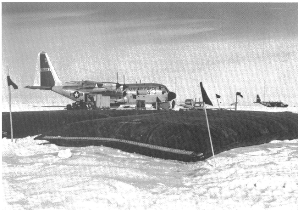
The U.S. Air Force introduced ski-equipped C-130As to antarctic service in 1960. Two fuel bladders are in the foreground.
