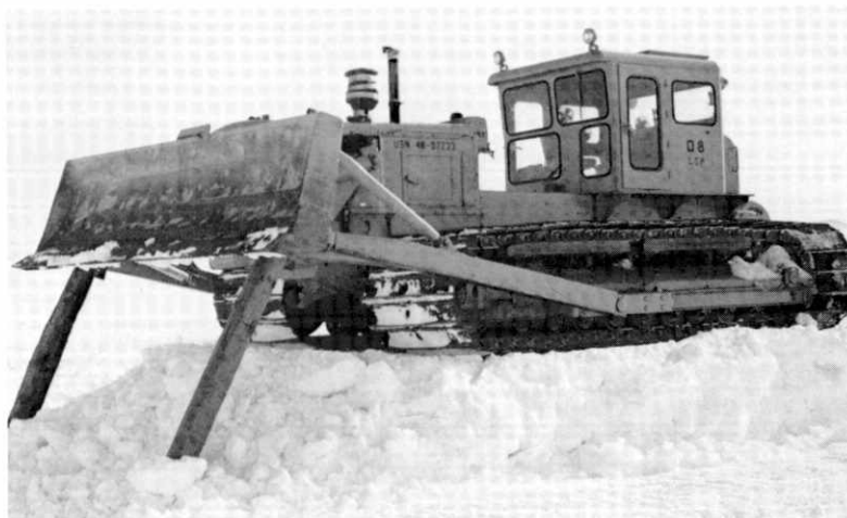
Figure 7. One of the original low ground pressure (LGP) D8 Caterpillar tractors used for traverses.
