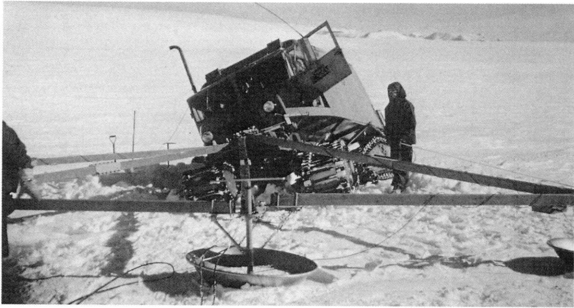
Figure 8. Tucker Sno-Cat (with device for crevasse detection mounted on front) in crevasse on Skelton Glacier in 1957.
