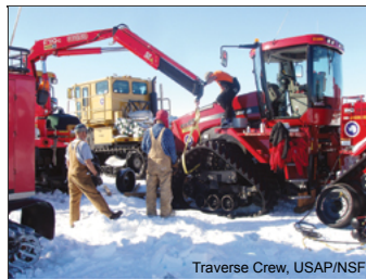
Traverse Crew, USAP/NSF Tearing down a drive track for a bearing replacement on the Leverett Glacier.
