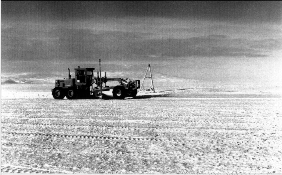
Figure 2. Laser-controlled grader used to level natural ice surface for runway.
