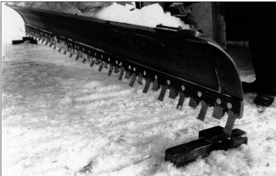
Figure 3. Custom-built grader blade for leveling glacial ice.
