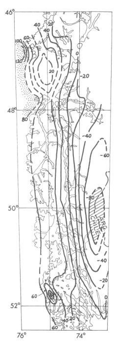
Figure 3. Generalized Bouguer gravity anomaly map of a portion of the southern Andes. Contour interval = 20 mgals. Areas with dots indicate values greater than +80 mgals; those with diagonal slashes indicate values less than -80 mgals.
